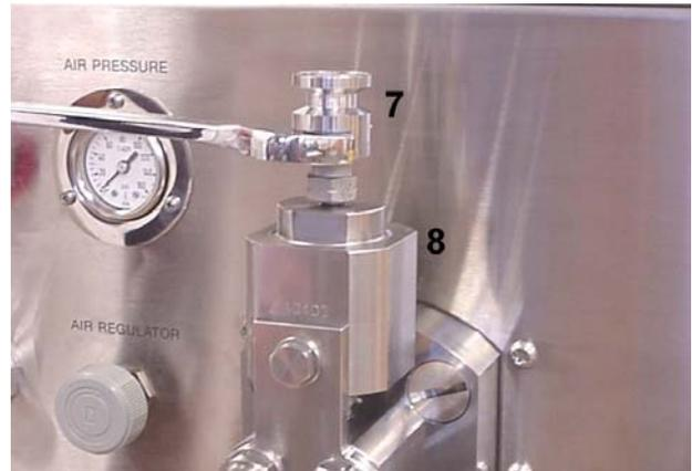
**Figure 7:** Removing an inlet fitting (7) from the inlet check valve (8). This inlet fitting is sanitary in design.
