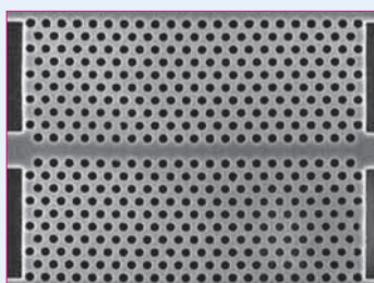
Photonic wave guide filter fabricated using mr-I T85, 320 nm deep holes transferred into silicon (200 nm diameter) (courtesy of MIC / TU Denmark)
