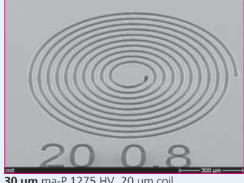
30 µm ma-P 1275 HV, 20 µm coil
