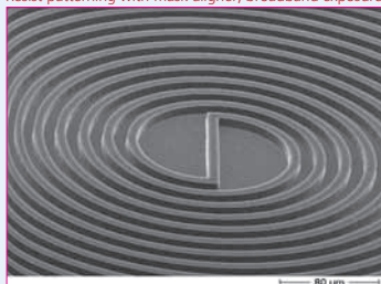
ma-P 1275, 7.5 µm thickness
