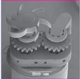
Windmill for fluidic media with a gearwheel connection
