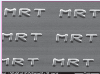
mr-UVCur06 mit UD15-Stempel G - 32. Imprint mr-UVCur06 structures (32 nd imprint with OrmoStamp)
