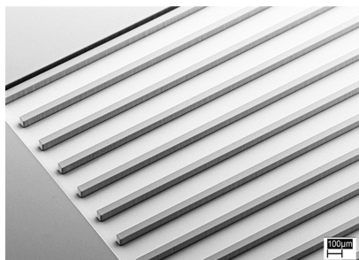
Fig. 4: EpoClad 50 x 50 µm structures on FR4 substrate
