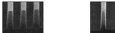
Dense and Isolated Lines/Spaces 0.325 \mu\text{m} Dense Lines/Spaces 0.250 \mu\text{m} Isolated Line
