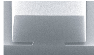
Figure 2. LOL2000 on Si at 200°C/5 min. with 5.0 micron SPR950
