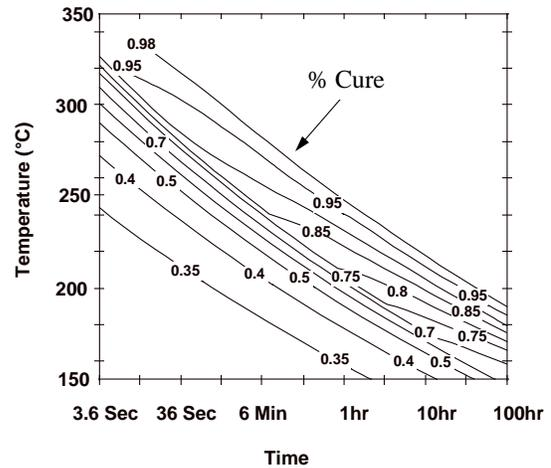
Table 12. Cure profiles for convection oven curing
