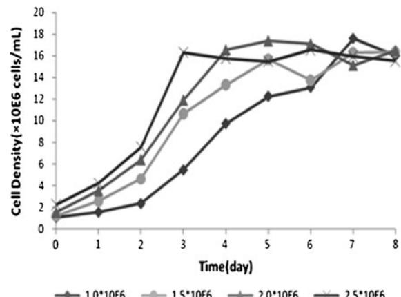
**Fig. 3** Effect of inoculation cell density on the growth kinetics of Sf-9 cells in TubeSpin bioreactors. The cells were inoculated at different starting cell densities as indicated. The cell density (a) and viability (b) were determined at the times indicated by manual counting using the Trypan Blue exclusion method. Each culture was performed in triplicate
