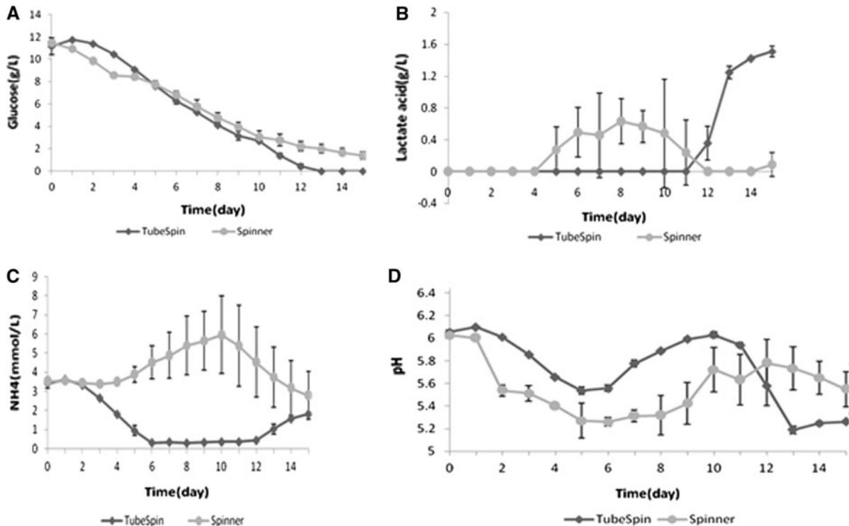
**Fig. 2** Comparison of Sf-9 cultures in TubeSpins and spinner flasks. The cultures were inoculated in duplicate at  $10^6$  cells/ml. Sampling was performed at the times indicated, and
