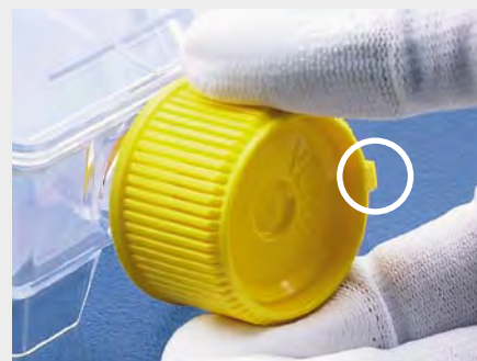
«VENT»-position at 3 o'clock = gas tight
