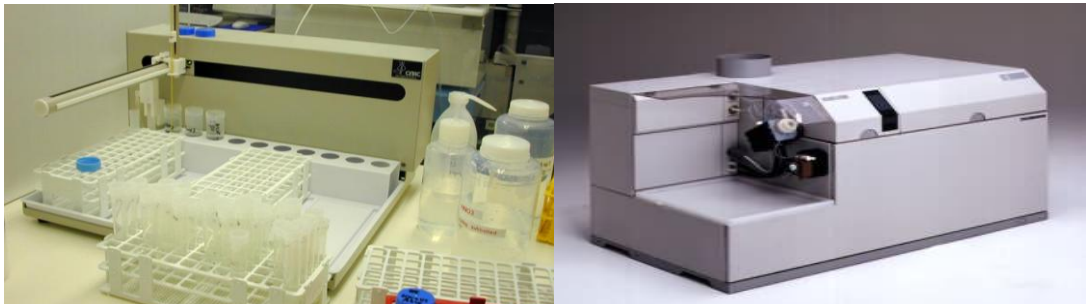
Figure3.(a) Autosampler (CETAC ASX-51 ). (b) ICP-MS (Agilent 7500a).
