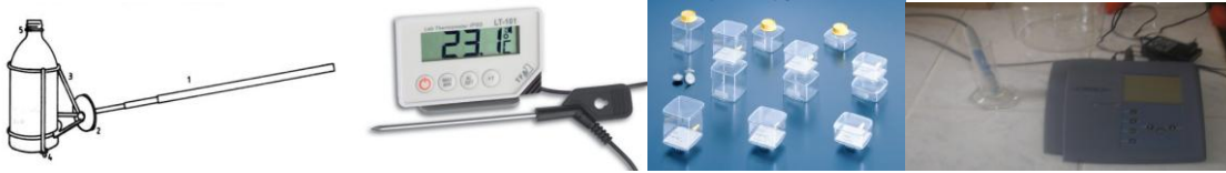
Figure2.(a) Equipment for sampling seawater (Mart, 1979). (b) TFA LT-101 Digital Thermometer. (c) TPP (Filtermax) Vacuum Systems. (d) WTW inoLab pH 720 Benchtop Meter.
