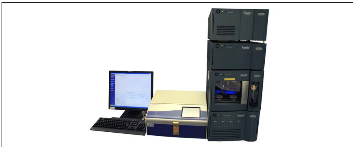
Figure 2: The radio-UPLC consists of the Waters Acquity UPLC™ System and the Berthold FlowStar LB513.
