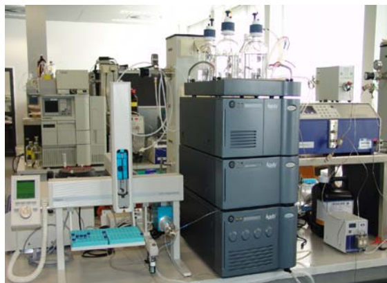
Figure 1. Waters Open Architecture UPLC® System coupled to Berthold online radioactivity detection.
