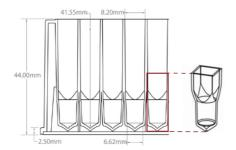
Each microwell is designed to fit the magnetic tips of all KingFisher™ purification systems using magnetic separation technologies.
