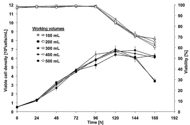
**Fig. 5.** Batch culture of CHO-IgG cells in a TubeSpin® bioreactor 600. The cultures were inoculated at  $5 \times 10^5$  cells/mL and grown at 37 °C with a shaking speed of 180 rpm at a range of different working volumes as indicated. The viable cell density (closed solid lines) and the percent cell viability (open dashed lines) were determined with the Trypan Blue exclusion method at the times indicated. Each experiment was performed in triplicate.
