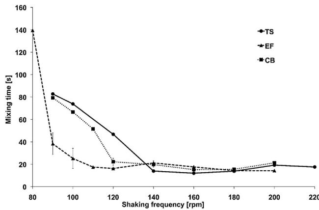
**Fig. 2.** Comparison of mixing time as a function of shaking frequency in OSRs. The mixing time values were calculated using DISMT. TubeSpin® bioreactor 600 (TS), 1-L Erlenmeyer shake flask (EF), and 1-L cylindrical glass bottle (CB) were filled with 300 mL of UHP deionized water at room temperature and orbitally shaken at various shaking frequencies. Each experiment was performed in duplicate.
